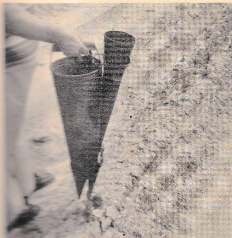
(4) Mechanism in your hand released the tobacco plant and some water at the same
